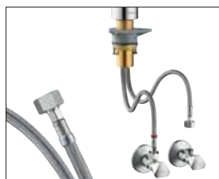
Safe, easy installation: Flexible connections and an integrated stabilisation plate make installation easier. The PEX hoses are temperature-resistant and neutral in taste and odour.
